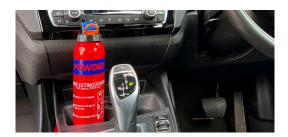
Where should powder be used? Less susceptible to freezing than water-based extinguishers, powder also suits outdoor storage and use, as well as being the standard for vehicle fire protection. This makes powder a great choice for keeping in your vehicle, garage, or home workshop. It is also ideal for caravans, camping, and small inland leisure boats.
